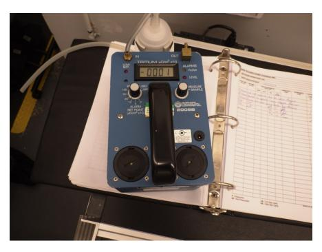
Figure 7. Portable Tritium In Air Monitor
